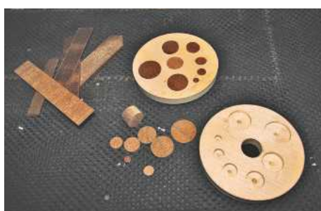
▲ Pic.5 On the outside of each wheel pencil a lazy S-shape and drill a series of holes of varying diameters
